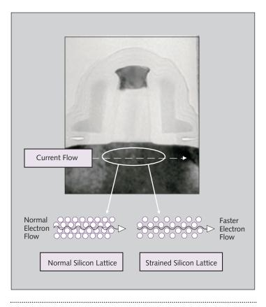
**Figure 1.** Strained silicon improves electron mobility by stretching the atoms in the silicon layer further apart.
