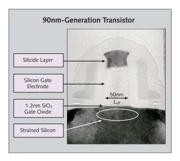
Figure 2. Intel's new transistors have some of the smallest features in the industry.
