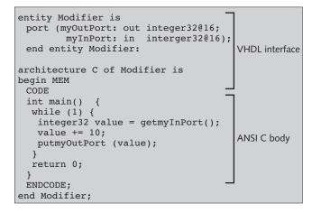
Figure 1. Programmers can specify the VHDL interface by using a structural subset of VHDL. The ANSI C bodies can use all features of C.
