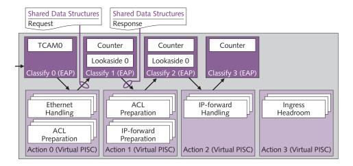
**Figure 1.** This flow diagram shows how the X10q pipeline handles the forwarding of Internet Protocol packets. Distributed throughout the pipeline are 11 engine access points (EAP) that manage programmed accesses to the function units, off-chip memory, and external coprocessors. The functions shown here would use about one-third of the X10q's 1,000-plus pipeline stages.
