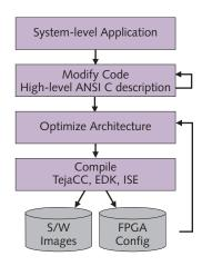
**Figure 3.** Hardware and software development with Teja FP is highly interactive. Using feedback from code profilers and actual execution in the target FPGA, developers can rapidly refine their design. The hardware/software partition is a movable wall: some operations that don't work well in software can be re-implemented in hardware, while other operations unsuitable for logic can be recompiled as software.
